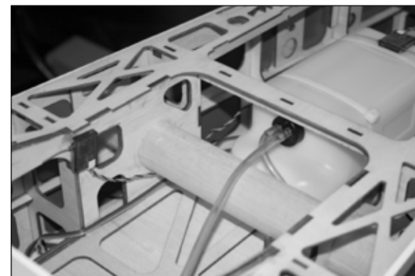
Location of Satellite receiver 4 - front of the tank and on the right vertical side.
