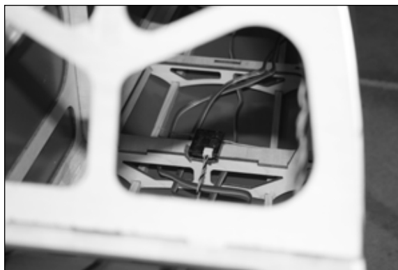
Location of Satellite receiver 2 - side of the fuselage tunnel.
