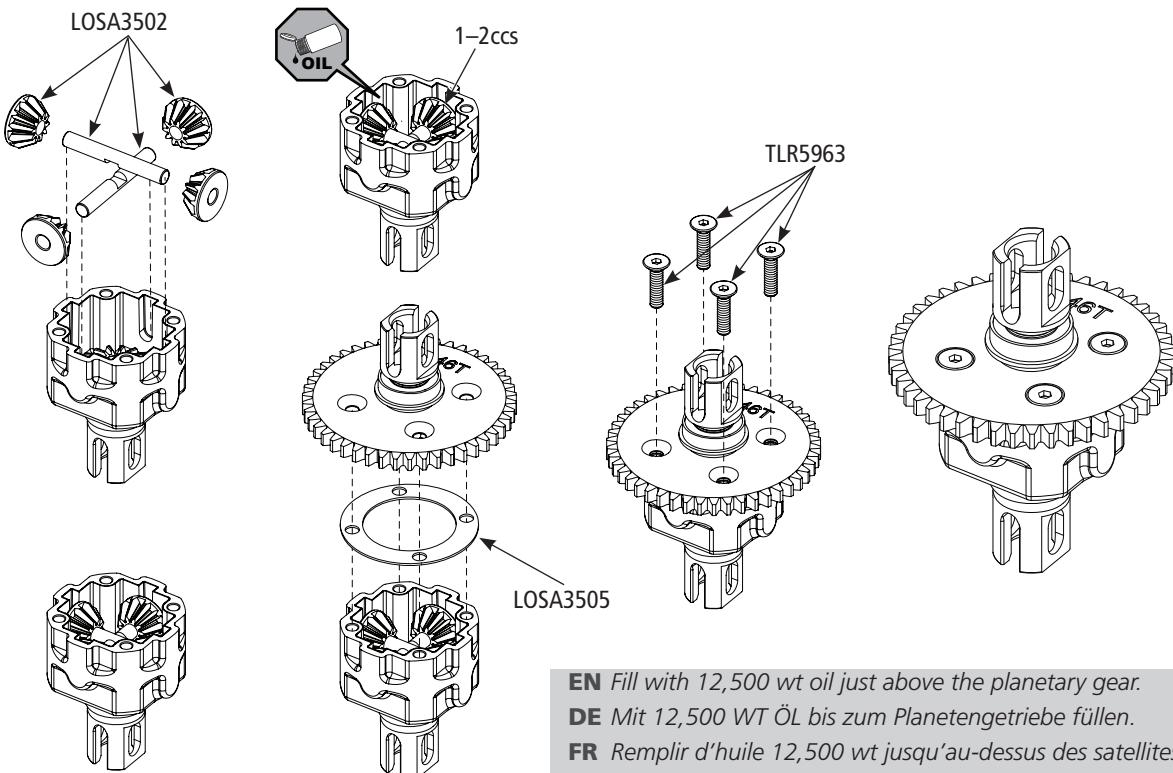
**EN** Fill with 12,500 wt oil just above the planetary gear.
