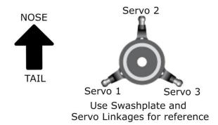
Using the Swashplate for reference. Follow the diagram here to trace the control linkage from the corresponding Swashplate arm down to the servo. A helpful tip, if you are having trouble, is to plug in a single servo into any of the 3 Servo Ports, power on the model, and see which one centers and moves. Using this procedure will help determine where each servo is located in reference to the swashplate diagram.
