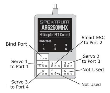
Once the servo location has been determined, use the receiver port assignment diagram to plug in the servos and Smart ESC.
