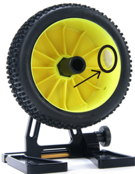
4. Spin the tire slowly to determine the unbalanced portion of the tire.
