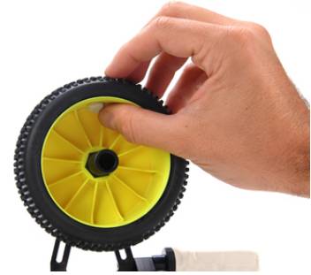
3. Insert the wheel nut into the spindle of the tire balancer and tighten.
