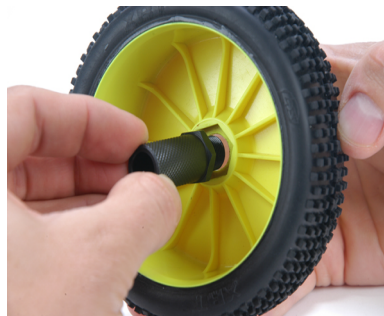
2. Insert the wheel nut into the wheel and lock the hex into place.
