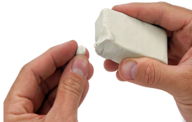
5. Remove a small amount of balancing clay to start balancing the tire. Prior to applying the balancing clay make sure the wheel is clean.
