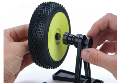
3. Insert the wheel nut into the spindle of the tire balancer and tighten.
