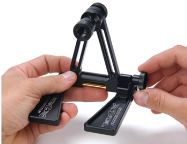
1. Insert the tire balancer handle into balancer arm and tighten.
