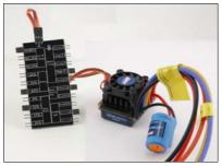
The Xcelorin Advanced Quick Programming Card (AQPC) is used to make all adjustments to the active profile in your ESC. Any ACTIVE profile can be modified.
