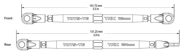
All of the toe links were originally installed on the truck so that the left hand thread indicators point in the same direction. This makes it easier to remember which way to turn the wrench to increase or decrease toe link length (the direction is the same at all four corners). Note that a groove indicates the side of the Tube with the left-hand threads.
