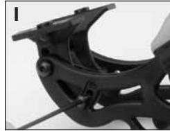
drilling the wing for proper hole spacing.
