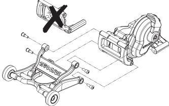
To install the #3678 wheelie bar on the Magnum 272R transmission, first remove the center mount from the wheelie bar by removing the four shoulder screws, and then secure the wheelie bar to the brace on the rear of the transmission case using the four shoulder screws. The additional hardware included with the #3678 package is not used.
