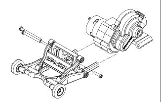
To install the #3678 wheelie bar on the Magnum 272 transmission, use the included hardware to secure the wheelie bar to the transmission case.
