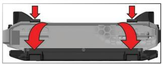
Install the battery pack with the battery wires facing the rear of the model.
