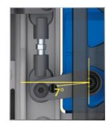
If necessary, fine-tune the length of the second steering link to eliminate any load on the steering system in the neutral position. If you are using aftermarket servos, it is important to use servo horns designed for E-Revo. Optional steering servo horns are sold separately for use with non-Traxxas servos.
