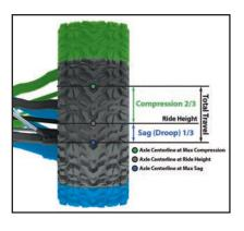
changing the position of the pushrods in the lower suspension arms. See the next section for ride height adjustments. The suspension sag and spring pre-load should be readjusted anytime the springs are removed and/or replaced.
