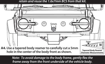
A5. Thread the wiring harness connector from the front LED light bar through the 5mm hole.
