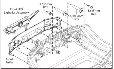
*Note: The 2.6x15mm BCS will break through the grille during installation.* Once the screws push through, clean away any plastic debris, and hold the light bar firmly against the grill while tightening the screws.
