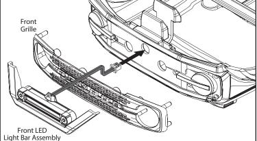
A6. Reinstall the front grille. Ensure that no wires are pinched between the vehicle body and the front grille before tightening screws.
