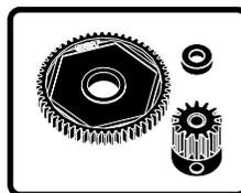
Inspect the spur and pinion gears for damage
