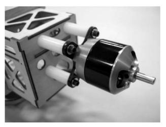
NOTE: Photo above shows installation using nylon motor standoffs.
