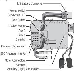
**NOTICE:** Always disconnect the battery from the ESC when you have finished operating your vehicle. If you leave the battery connected with the power switch in the OFF position, the ESC will continue to draw current when connected to the battery, resulting in possible damage to the battery through over-discharge.
